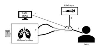
Figure 1 - Example of the assembly and arrangement of sedation equipment with volatile agents in the intensive care unit.
